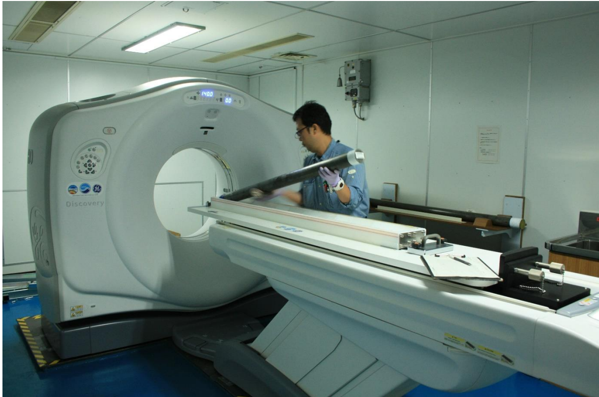
Figure 3. Technician Soichi Moriya preparing a fresh core for the 3D X-ray CT scan.
